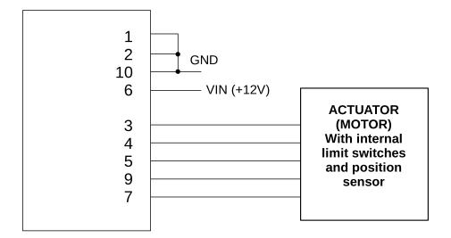
**ATTENTION!** Always refer to the documentation for the actuator used to identify the appropriate signals for the motor and position sensor. Then connect to the corresponding pins of the control unit connector, which are described in the table in chapter 4.4.
