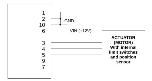
**ATTENTION!** Always refer to the documentation for the actuator used to identify the appropriate signals for the motor and position sensor. Then connect to the corresponding pins of the control unit connector, which are described in the table in chapter 4.4.
