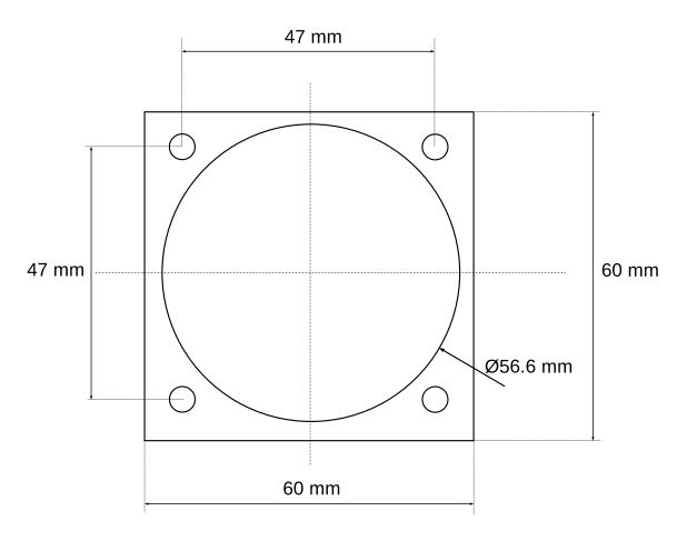
Mounting holes are provided with M3 thread and 4 mm thread depth.
