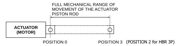
Observe the following points when installing the actuator:
