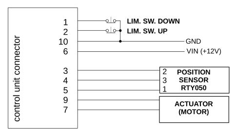
**ATTENTION!** Always check with care that the actuator moves the flaps in the intended direction and not vice versa. If it moves the other way around, the motor wires are probably swapped. This test should be performed WITHOUT a connected position sensor, when the control unit enters Safety (manual) mode and therefore this test will not be affected by a potentially inverted position sensor (which is second option what coud be wrong).
